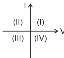
A. For a solar-cell, the I-V characteristics lies in the IV quadrant of the given graph.
